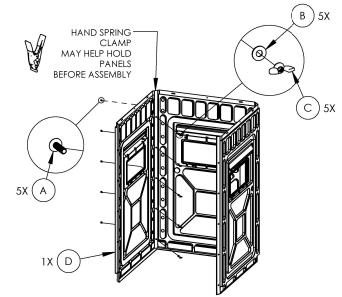
STEP 3: STAND THE DOOR PANEL "E" AND ALIGN THE SCREW HOLES TO CLOSE THE LAST CORNERS. INSERT (10) SCREWS "A" THROUGH BOTH PANELS FROM THE OUTSIDE OF THE BLIND. FASTEN EACH SCREW WITH A WASHER "B" & WING NUT "C".
